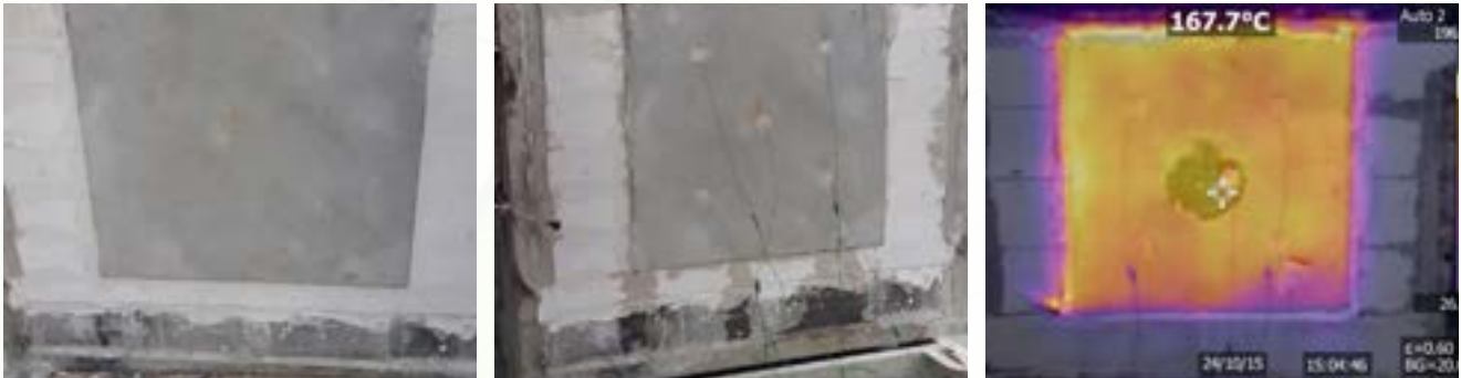
Figure 12. Fire resistance test (PCE1)
