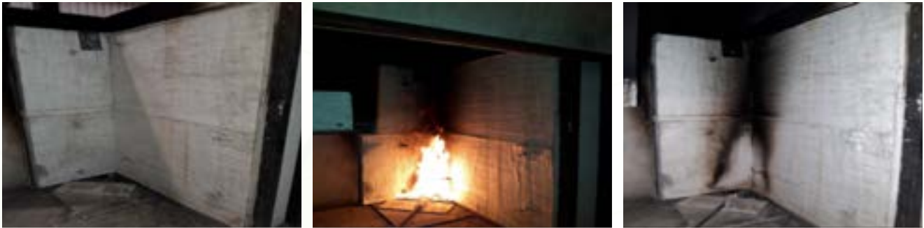
Figure 15. Fire reaction test (aerogel surface)
