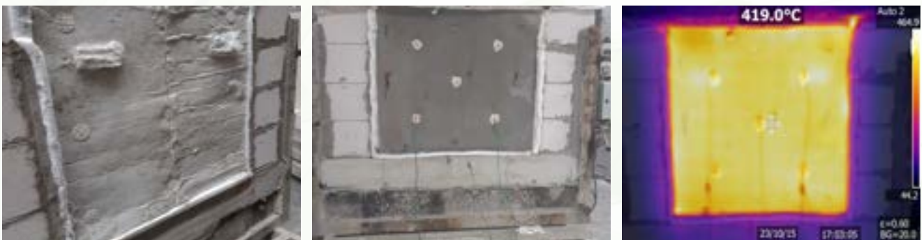
Figure 13. Fire resistance test (PCE2)
