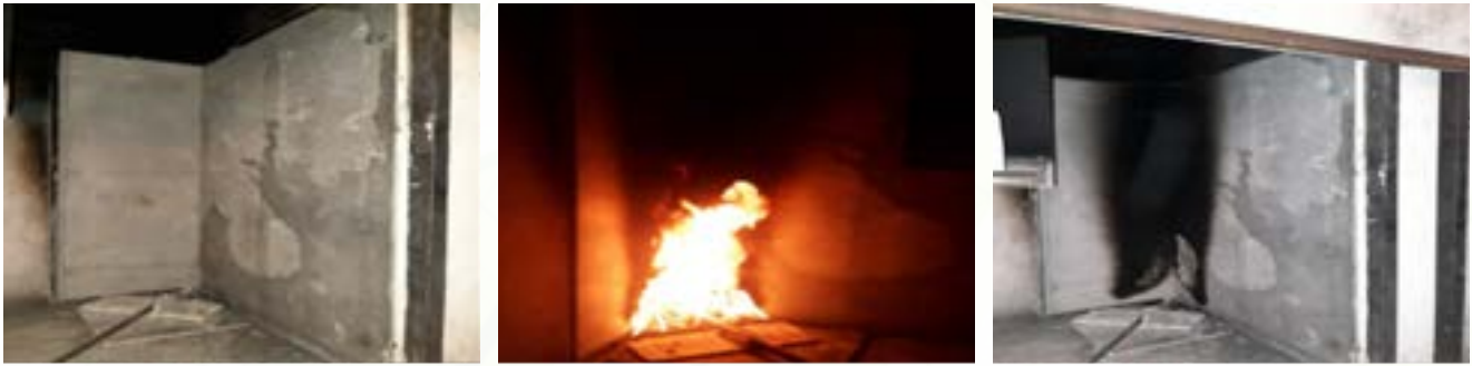
Figure 14. Fire reaction test (concrete surface)
