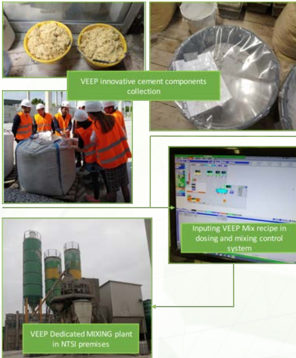
Figure 8. VEEP PCEs concrete main production phases
