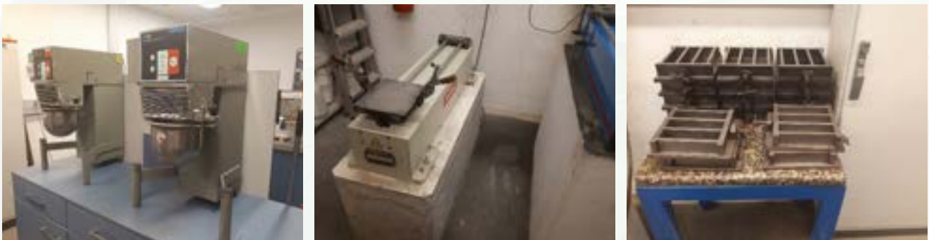
Figure 1. Laboratory equipment for the manufacture of standard mortars and cement control @Tecnalia laboratory
