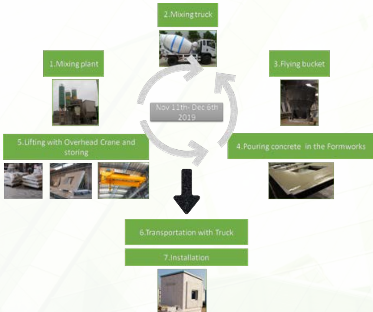
Figure 9. VEEP PCEs advanced manufacturing cycle
